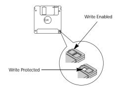
Figure 4-3 Floppy Disk Write Protect
